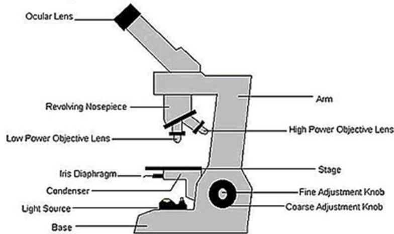
Parts of the Microscope
